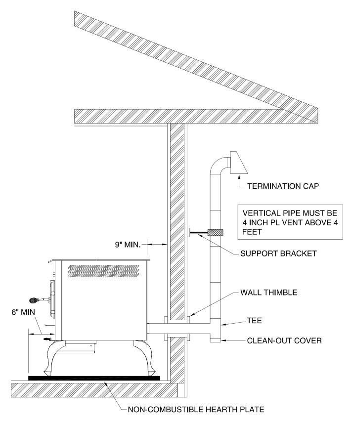
The Hearth Pad is not required under the unit if the floor is noncombustible but is required 6 inches (152mm) beyond the front of the unit and 6 inches (152mm) beyond each side of the door if the floor is a combustble floor. wood flooring, carpet, linoleum, etc.
